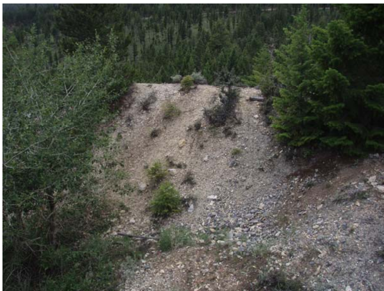
Photo #39 Waste Dump developed by excavation of the Gilmore Mine Adit and Decline.(B. Schuld 7/22/10)
