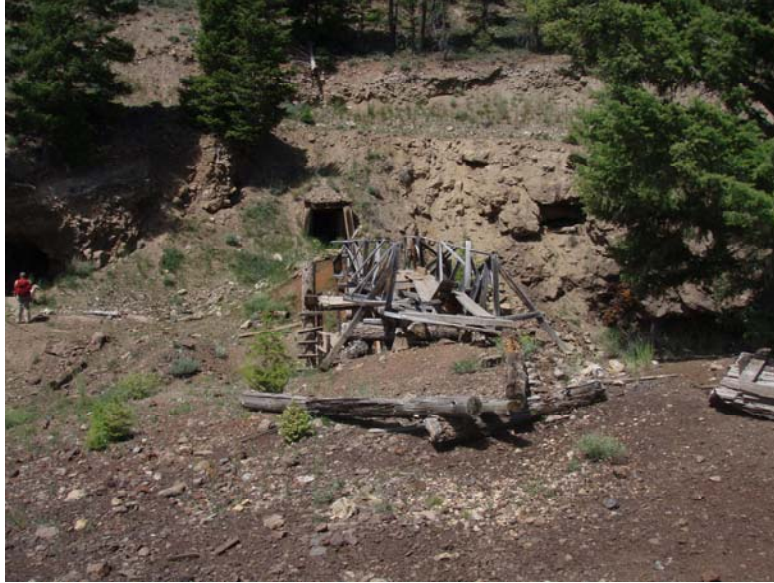
Photo #23 Three dangerously open adits remain on the Silver Dollar. There as apparently some redevelopment work that was conducted on these adits and a small ore bin/chute was constructed to ship some ore or samples. (B. Schuld 7/22/10).
