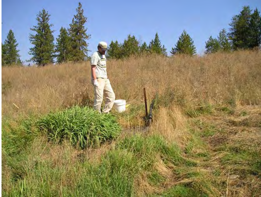
Figure 9. Photo taken September 2, 2006 showing discharge pipe for water park back flush water. Discharge was measured at 16 gallons per minute.
