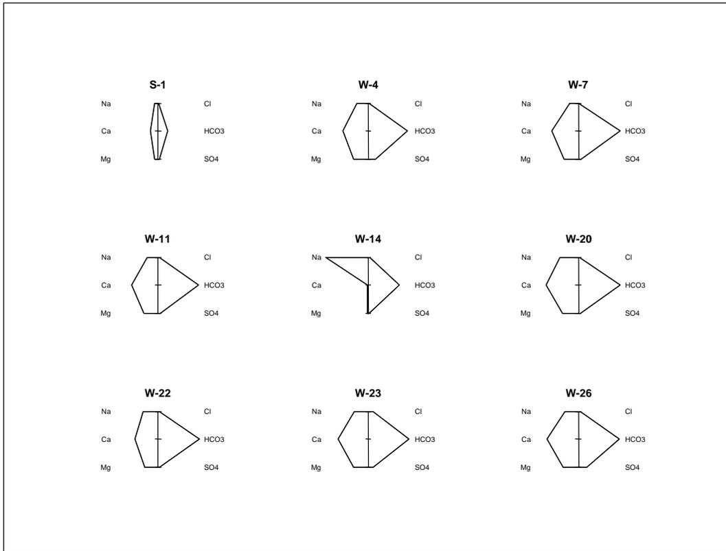
Figure 8. Stiff diagrams showing cation and anion concentrations, in millequivalents per liter, for 9 selected spring and well samples in the Cow Creek drainage.
