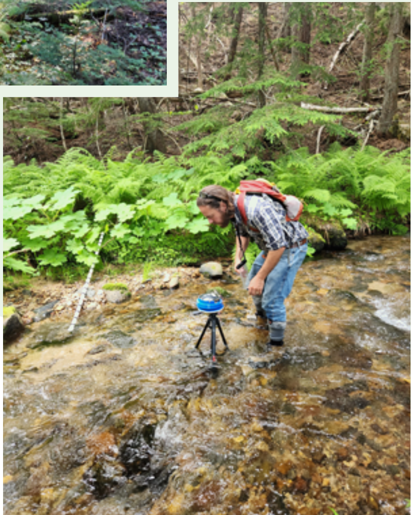
Figure C19. Measuring shade using a Solar Pathfinder.
