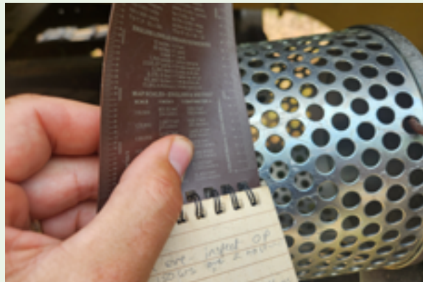
Figure C13. Measuring a water screen.
