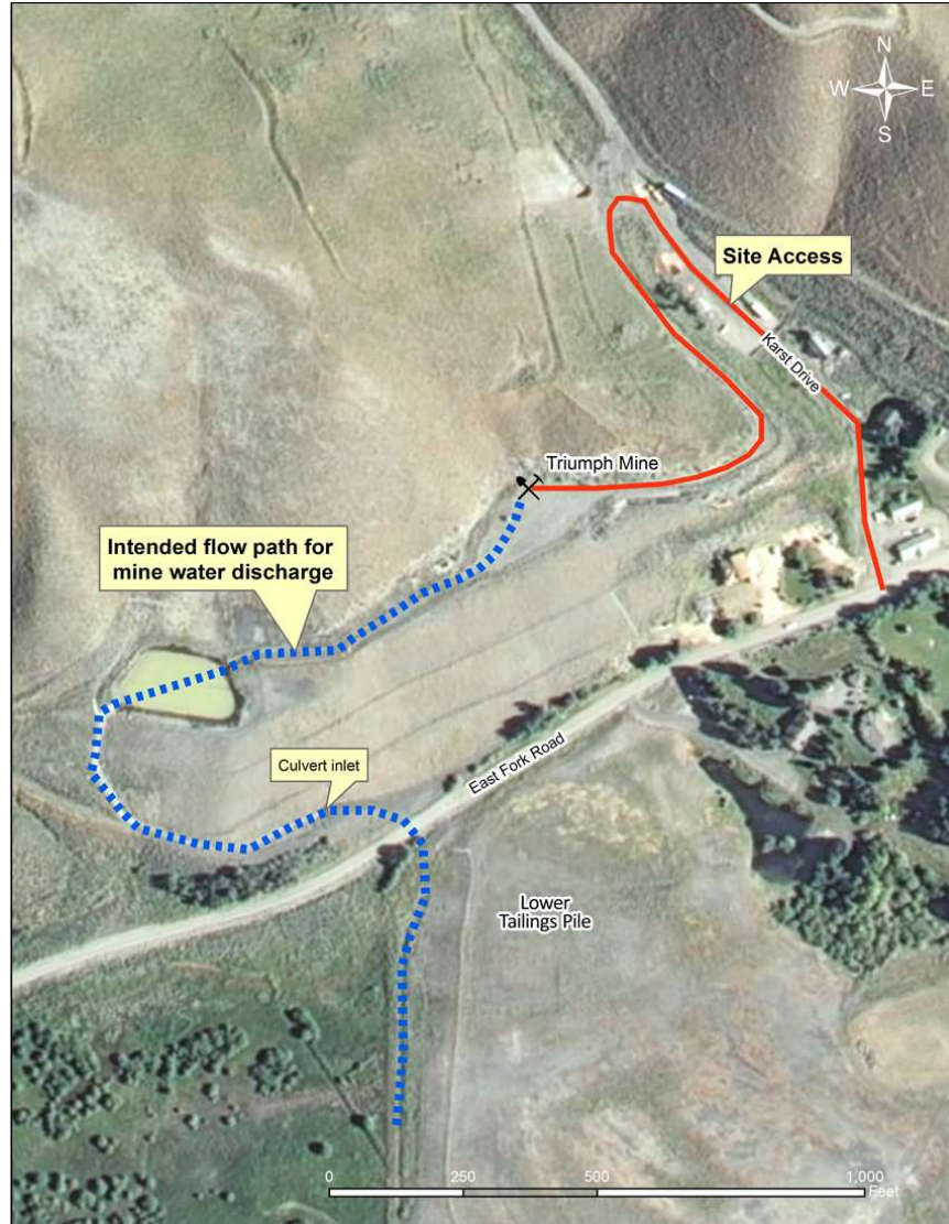
Figure 2. Triumph Mine site access and intended flow path for mine water discharge.
