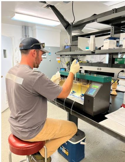
Initial jar testing for metals and phosphorus
