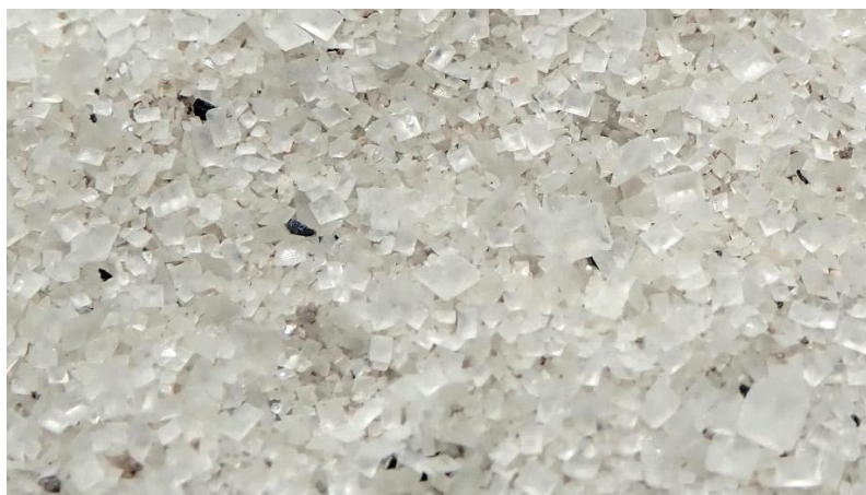
Figure 1: Struvite harvested by the MagPrex system under controlled conditions
