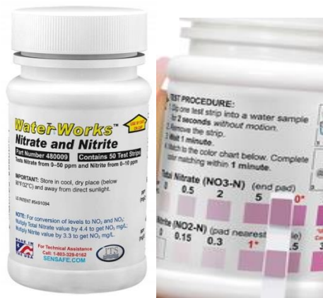
Figure 16. Images of WaterWorks™ Nitrate and Nitrite test strips and method of results interpretation.
