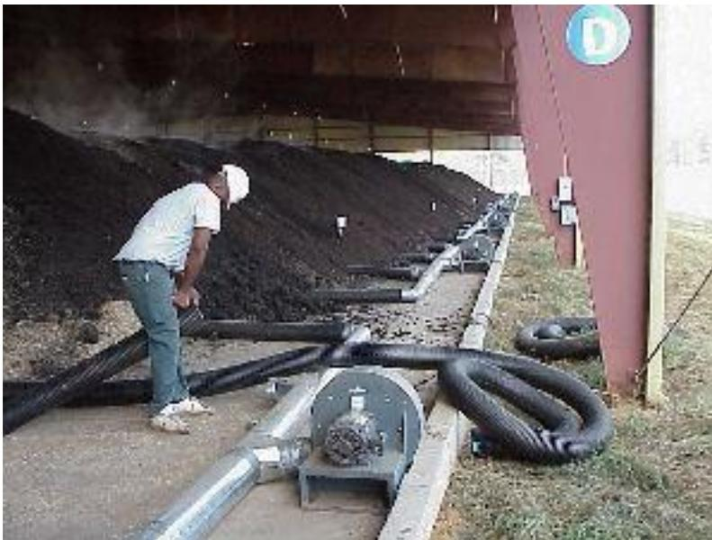
Figure 2. Aerated static piles (photo courtesy of the University of Idaho).
