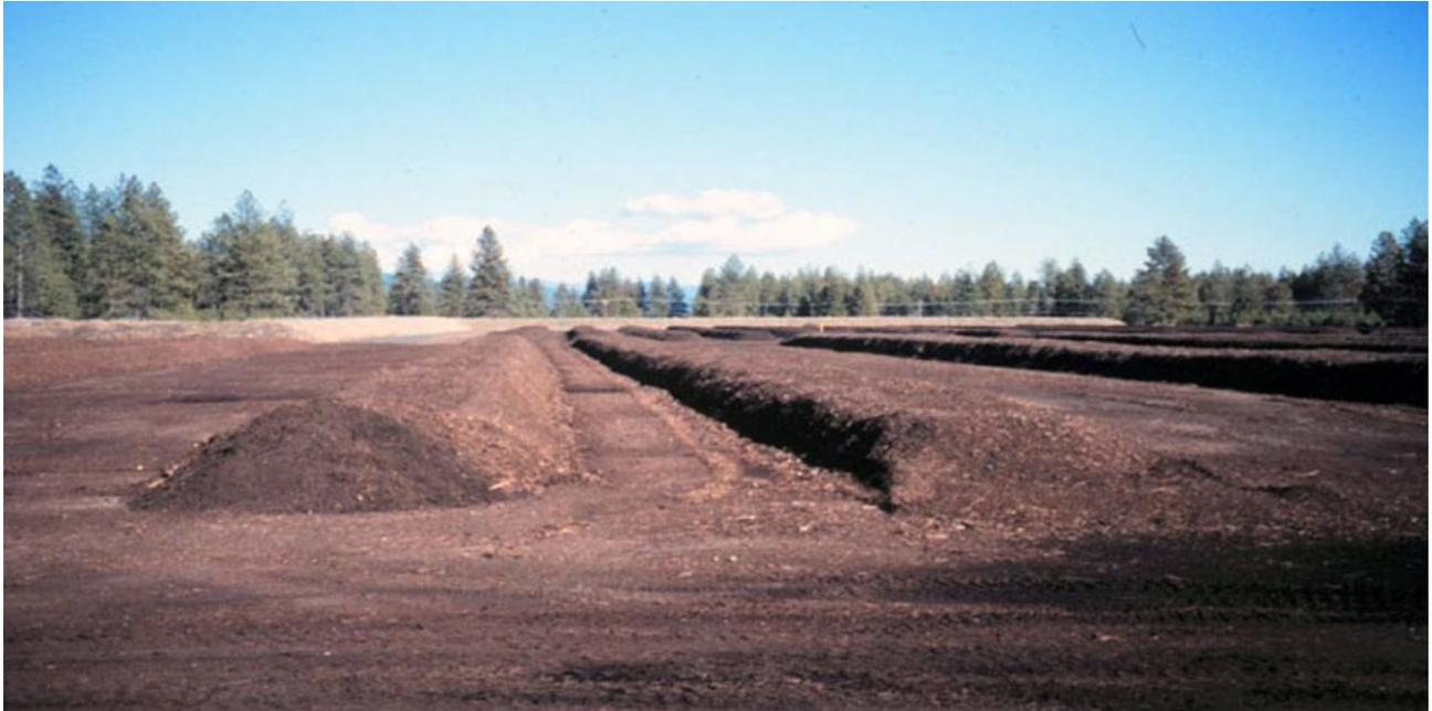
Figure 1. Windrow composting (photo courtesy of Washington State University).
