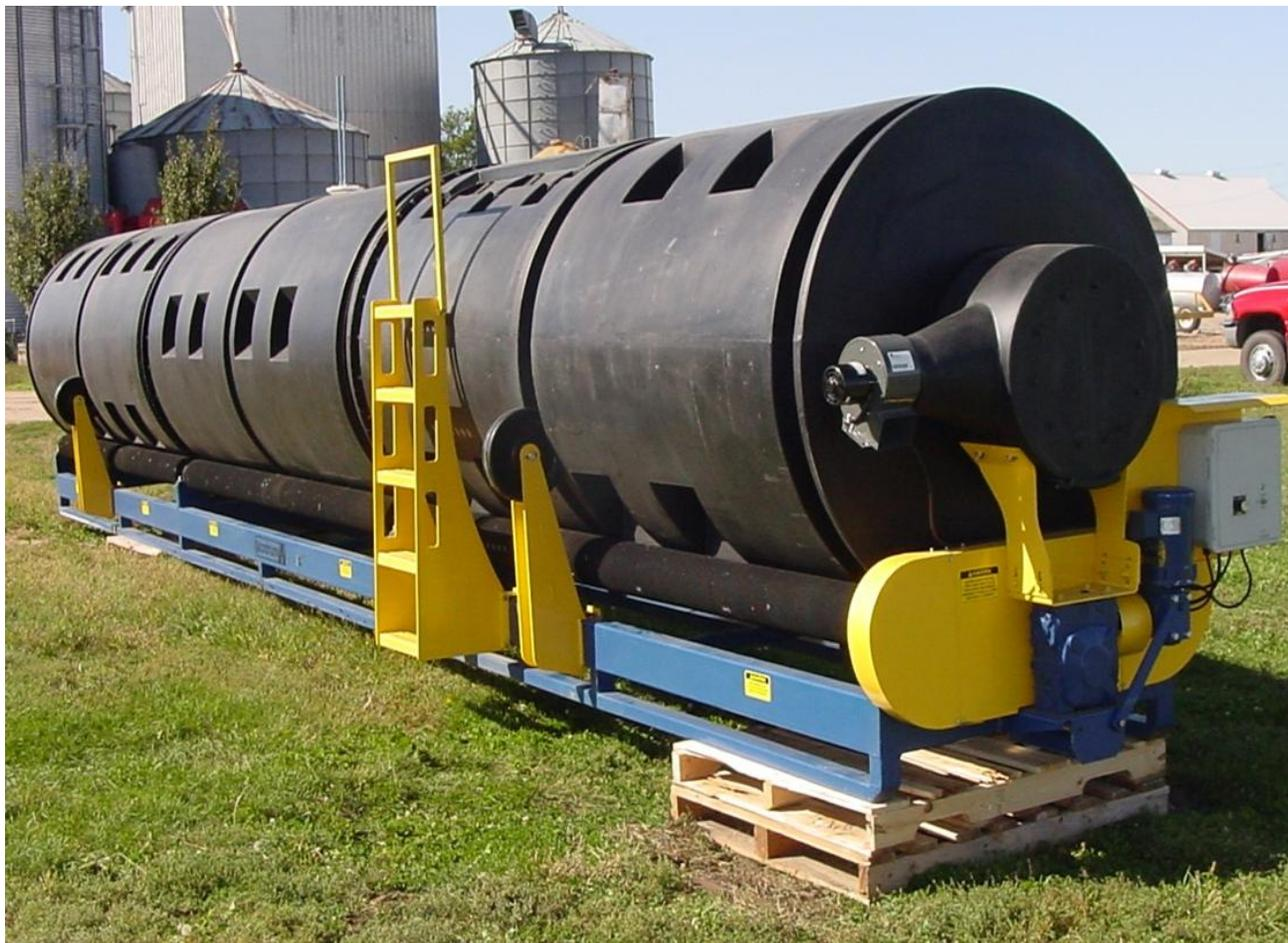
Figure 3. In-vessel composting (photo courtesy of Duke University).
